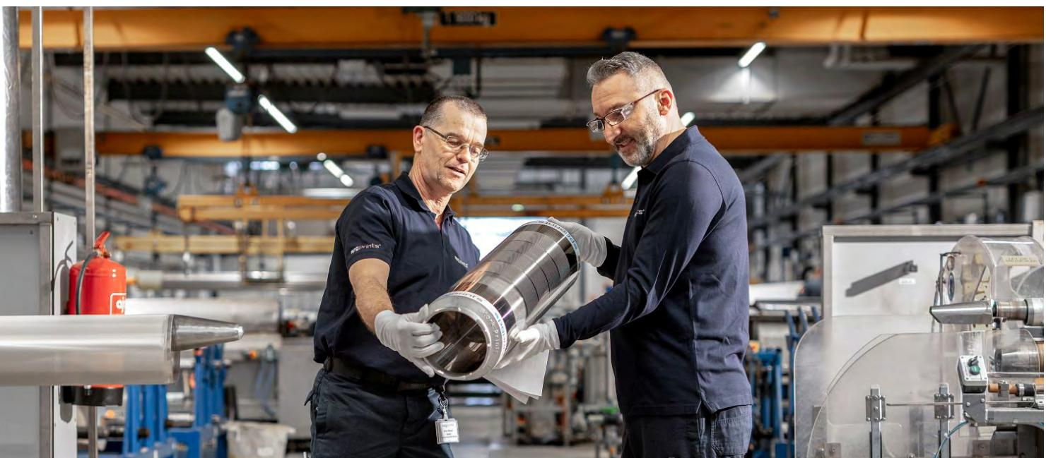
To produce non-woven fabrics, a popular production method is hydro-entanglement. The screens used during manufacturing play a vital role during the hydro-jetting process in determining the effectiveness of this entanglement. The screens play an important role in dictating the quality and consistency of the finished product.
